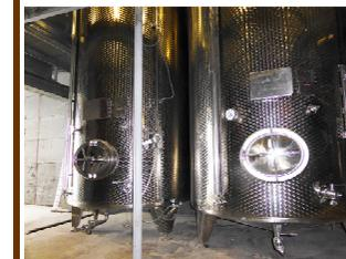
They are from electropolishing stainless steel which makes cleaning simple. The thermal insulation allows assisting the fermentation more precisely and limits the electricity consumption. The floating tank lids make it easier to manage the volume.
